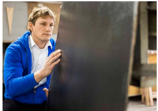
Visually inspecting a carbon-reinforced surface (Image: HA Hessen Agentur GmbH - Jan Michael Hosan)
