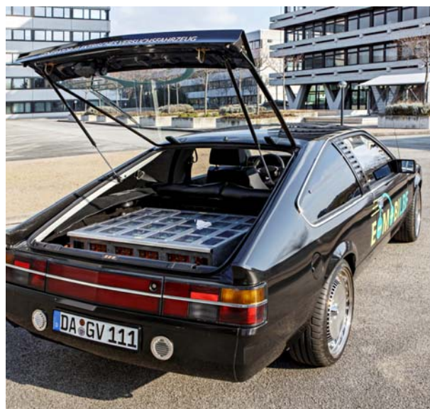
The Fraunhofer LBF's concept vehicle, featuring a 10 kWh LFP battery and an integrated battery management system
