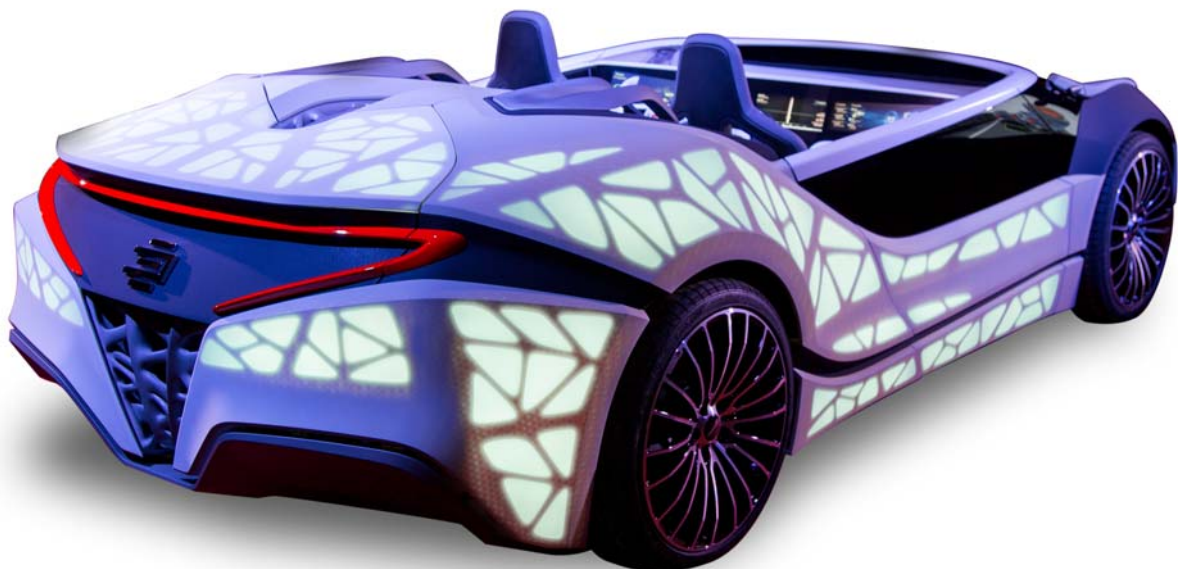
Image 4: The design engineers took nature as their inspiration by using a tortoise shell as the blueprint for the development of the concept car EDAG Soulmate (2016). (Image: EDAG Engineering GmbH)
