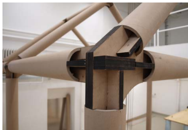
Cross structure for connecting paper sleeves for framework structures
