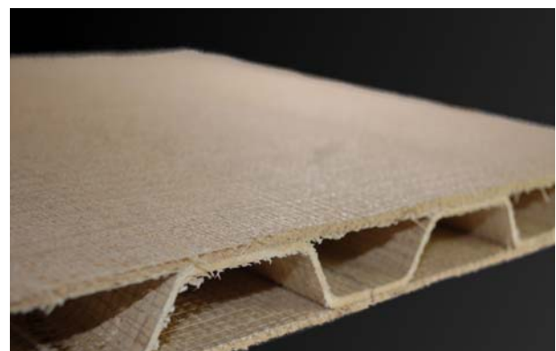
Sandwich structure made of flax-fibre reinforced paper
