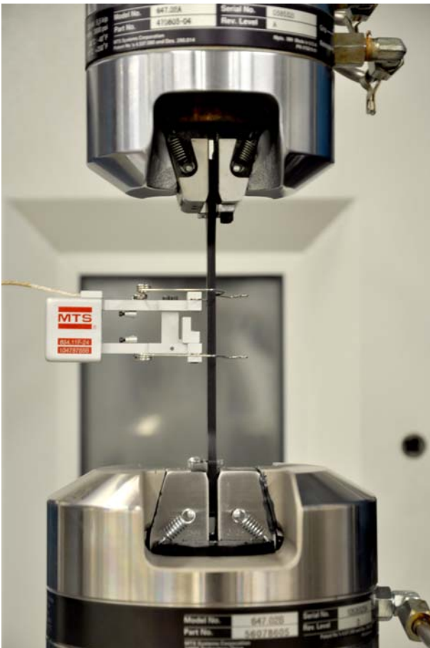
Cyclic-dynamic material testing of short fibre-reinforced plastic
