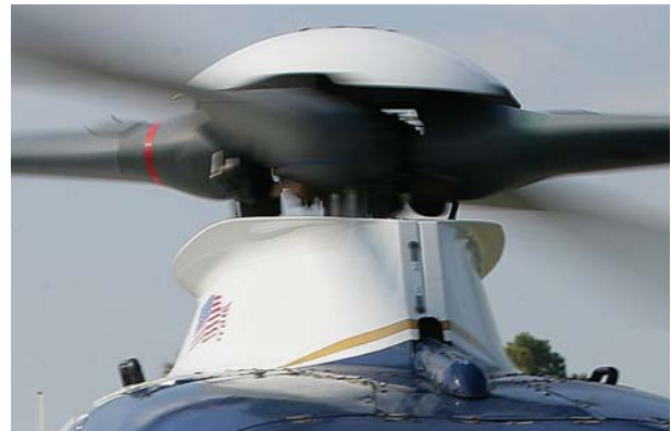
Image 5: Lightweight design through function integration - bearing and hingeless rotor system of the Airbus helicopter H135 (previously EC135, below) compared to a fully hinged rotor system. (Image top: "Airbus")
