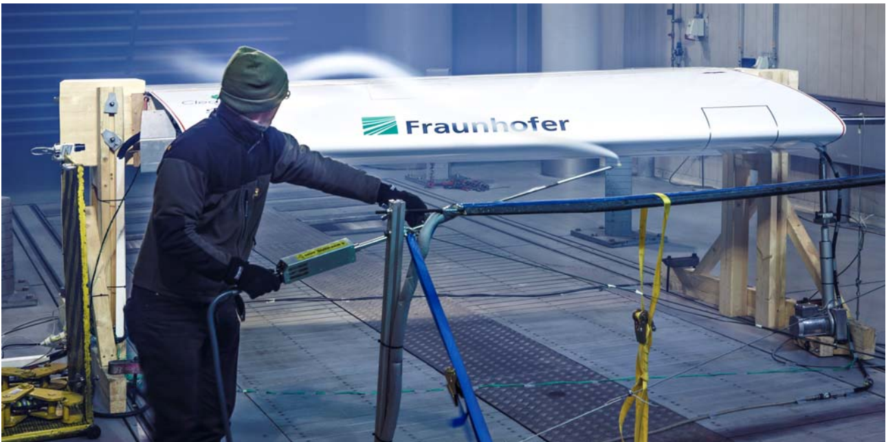
EU JTI CleanSky wing demonstrator with a shape variable front edge in a wind tunnel
