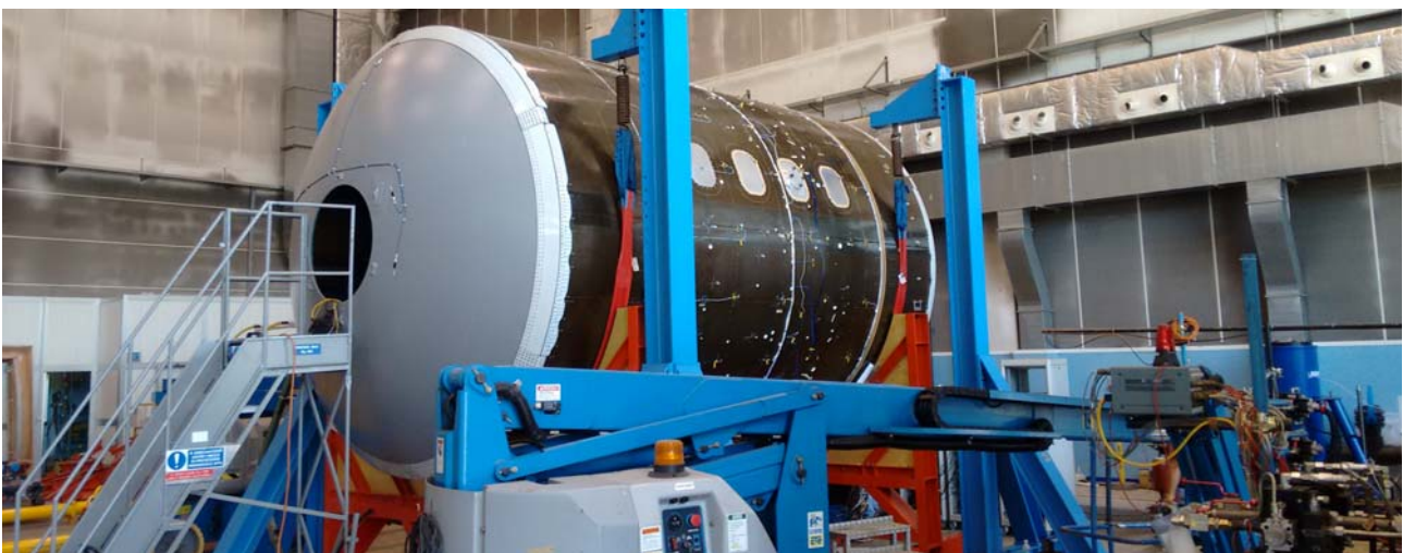
Ground test in the laboratory: A special measurement setup detects the cyclic internal pressure load on an aircraft fuselage simulated by inflation. (Image: ©Leonardo)
