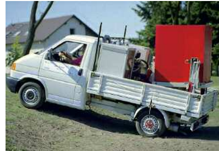
Adaptronic transportation system for maintaining the position of a transport medium [© Fludicon GmbH]
