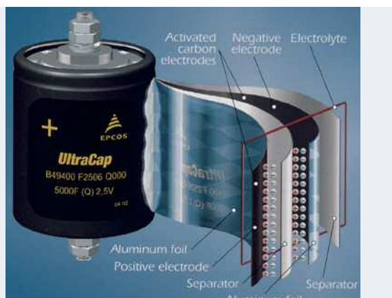
Set-up of a super capacitor [© EPCOS AG]
