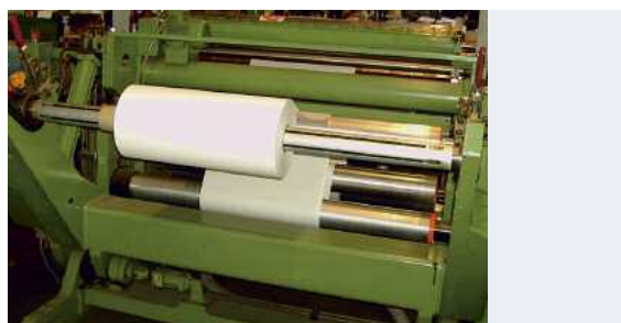
Paper produced by the special paper manufacturer Oberschmitt GmbH for operation as separator material in super caps. The main advantage of the paper is its fine and dense structure with simultaneous good permeability for the electrolyte.
