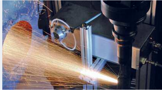
Preparation of the engine block for nano coating (left) and coating of the engine block (right) [© DaimlerChrysler AG]
