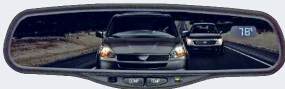
Effect of electrochromic coating demonstrated by the example of a rear view mirror [© Gentex GmbH]
