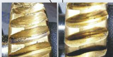
Nanostructured wear protection layers for machine components with a high mechanical load (e.g. engines, bearings, drilling equipment)
