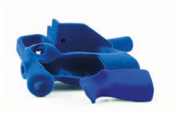
Laser-sintered handles of the Nikon Metrology Scanner with flocking (Source: Materialise)
