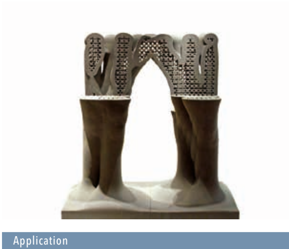
Printed architectural columns with internal cavities infiltrated with sand and epoxy resin (Source: Daniel Büning)
