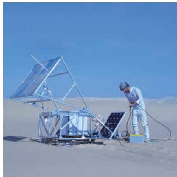
The German designer Markus Kayser with his solar sintering system at work (Source: Markus Kayser)
