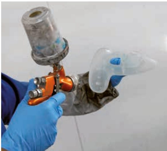
Transparent finish of a stereolithography component (Source: Materialise)
