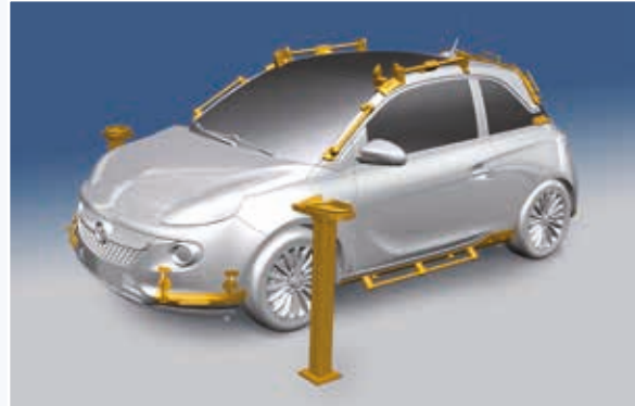
Design and modification of the assembly tools carried out on the computer (Source: Adam Opel AG)
