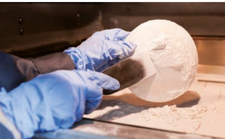
Component removal from the powder bed (Source: Evonik Industries)
