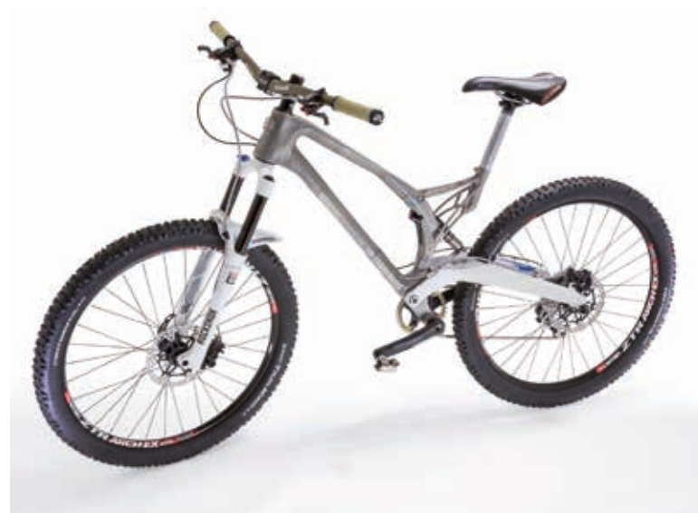
Not yet motorised but a pioneering role on the path toward a completely additively manufactured chassis: in February 2014 the first bicycle frame was presented which was manufactured out of a titanium alloy exclusively using additive processes. (Source: Renishaw)
