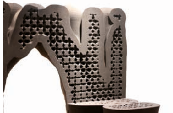
Natural Column and the hollow interior structure (Source: Daniel Büning)
