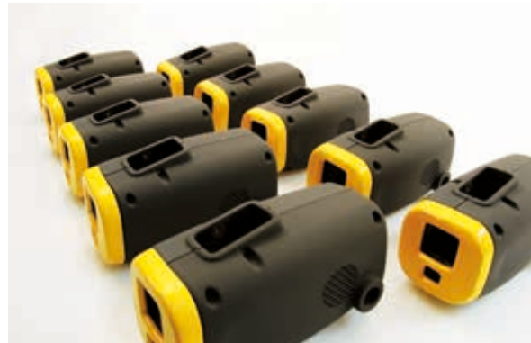
Housing produced from an additively manufactured master form for a hand scanner from Nikon Metrology (Source: Materialise)
