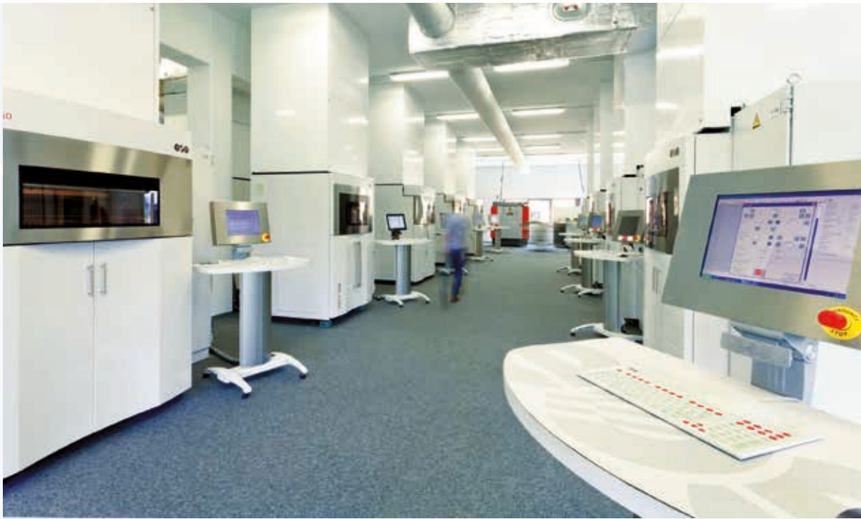
Manufacturing hall with 25 laser sintering systems and automatically controlled material cycles (Source: FKM Sintertechnik)
