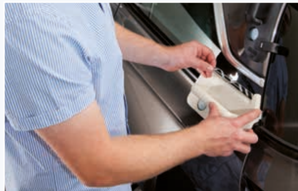
As part of the production of the Opel ADAM ROCKS an assembly aid manufactured via a 3D printer is used to attach the vehicle lettering to the rear side windows, for example. (Source: Adam Opel AG)
