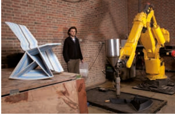
endless flow – robot-guided extrusion printing (Design: Dirk Vander Kooij)
