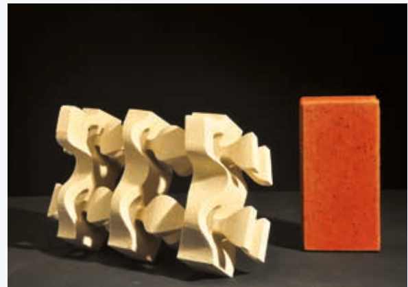
Prototype of a parametric module without formwork (Source: University of Kassel, J. Frankenstein-Frambach, A. Fromm)
