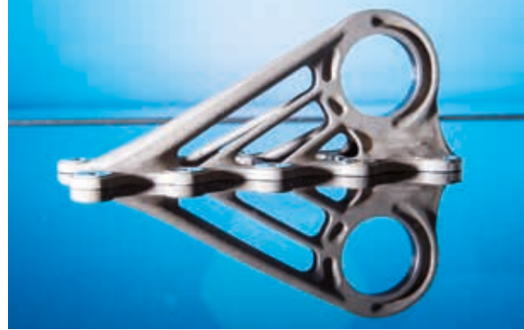
Titanium connecting element for the Airbus A350 XWB generated using laser melting (Source: Airbus, Laser Zentrum Nord)
