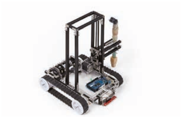
Minibuilders robots for creating printed architecture (Source: IAAC, Barcelona)
