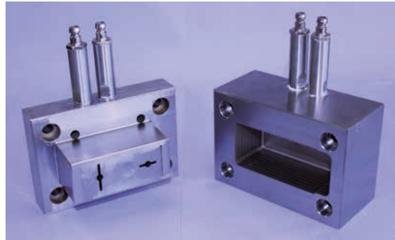
Toolpiece manufactured using plate press brazing (Source: Neue Materialien Bayreuth GmbH)
