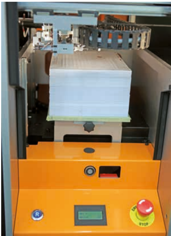
Construction space of a MCor system after the layer lamination process (Source: 3D-Picture, photo: Dieter Bielert)
