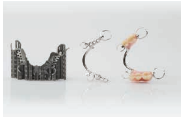
Manufacturing steps of a laser-centred model casting prosthetic: Dental prosthetic immediately after the manufacturing process, support structures removed and surface polished, after completion (Source: EOS)
