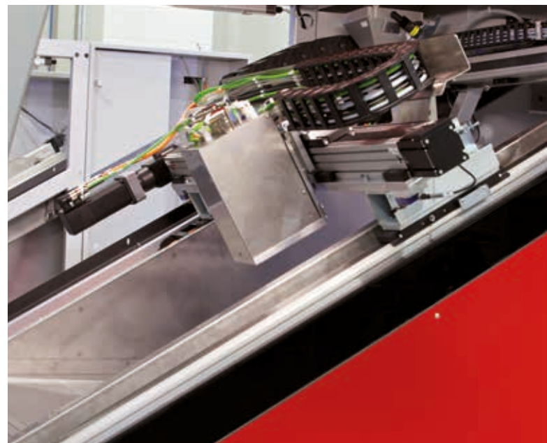
VXC800: Continuous 3D printing with an inclined printing bed (Source: voxeljet)
